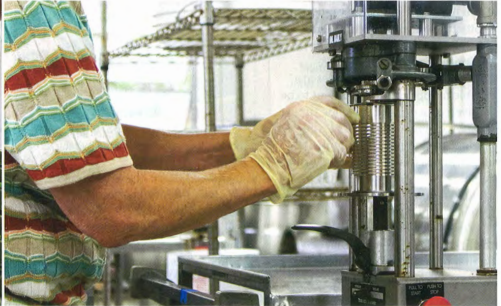
Cans are double-sealed with the cannery's seamer.
