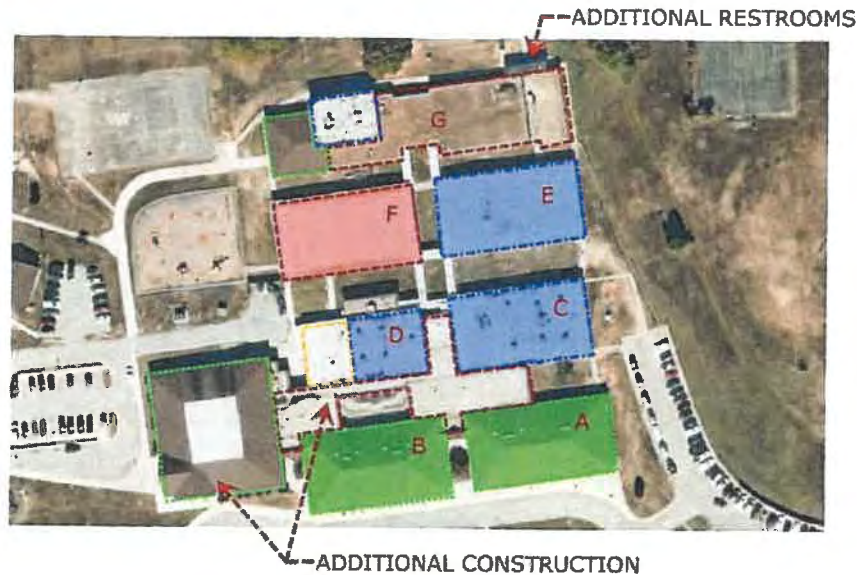
Pictured above: Ballasted Membrane Roof in Red. Membrane roof (coated) in Blue. Sloped roof in Green. Modified bitumen roof in yellow. Shaded areas indicate existing concrete double tee structure. Building designations indicated in red.
