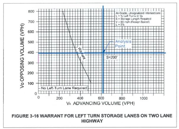
Current traffic requires a 200' full width left turn lane with a 200' taper, but Maxey & Associates, P.C. recommends that the full width left turn lane be extended to 350' to accommodate future development.
